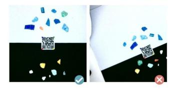
Particles should be carefully placed on the background sheet. Place light particles on the black half of the background sheet and dark particles on the light half to increase contrast.
