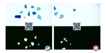
Ensure no particles are overlapping. If particles overlap, they will be detected as a single particle, which will lead to inaccurate results.
