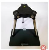
Do not image particles without shroud in place.
